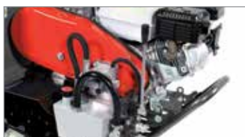
Lever-operated hydraulic tipping control valve.
