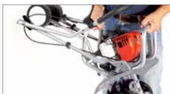
Folding handlebars for easy storage and transport (e.g. in the boot of a car).
