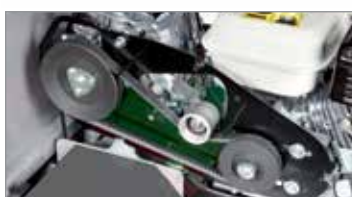
Belt clutch with automatic disengagement when the control lever is released.
