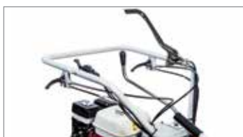
Steering with independently controlled releases and brakes.
