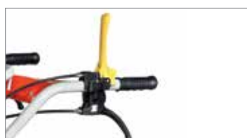
Handlebar-mounted gear selection lever.
