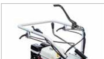
Steering with independently controlled releases and brakes.
