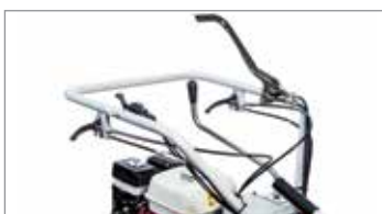
Steering with independently controlled releases and brakes.
