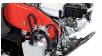
Lever-operated hydraulic tipping control valve.
