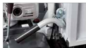
Manual dump with automatic locking system.
