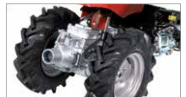
Integral QuickFit coupling that allows the operator to change the tools without using tools.
