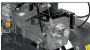
Direct gear transmission on crankshaft.
