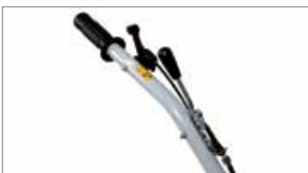
Handlebar-mounted PTO control.
