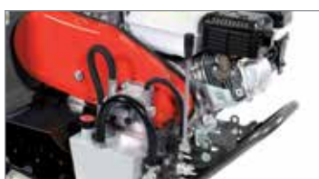
Lever-operated hydraulic tipping control valve.
