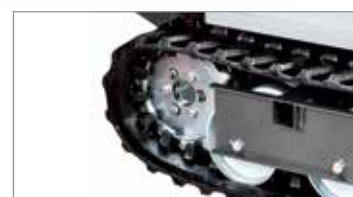
Protected, expandable brakes for working in extreme conditions.
