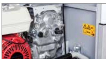
Independent PTO at 2100 rpm.
