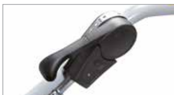
Handlebar-mounted PTO control.
