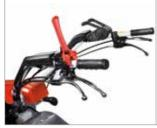
Easy reachable commands: brakes can be activated separately, handlebar unlocks and rotates 180°, thus allowing to maneuver the machine on most difficult terrains (KAM 7 S, KAM 13 S).
