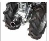
QuickFit coupling that allows the operator to change the tools without using tools (optional).
