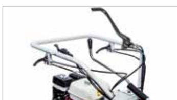
Steering with independently controlled releases and brakes.
