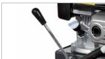
Speed selection control lever.
