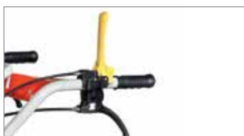
Handlebar-mounted gear selection lever.
