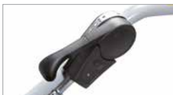
Handlebar-mounted PTO control.
