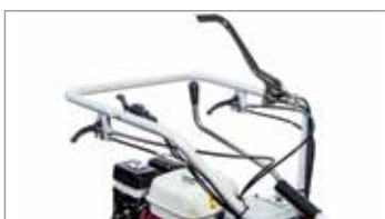
Steering with independently controlled releases and brakes.
