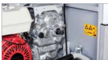
Independent PTO at 2100 rpm.
