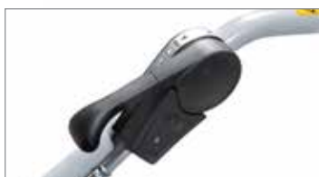
Handlebar-mounted PTO control.
