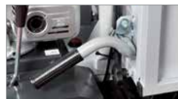
Manual dump with automatic locking system.
